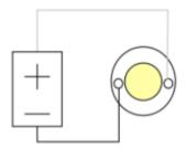
There are four different ways to set it up to light the bulb. Switch the wires for two of the ways to light the bulb, switch the battery around for the other two.
